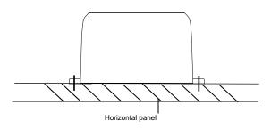
For best results, the rain sensor should be securely mounted onto a horizontal surface about 39.37" (1 meter) above the ground (or higher) and in an open area away from trees or other coverings where rainfall may be reduced causing inaccurate readings.
